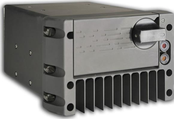
Fig. 10 The VS1410 On-board mission recorder implementing the pipeline described in this work over a total of 2W of power
