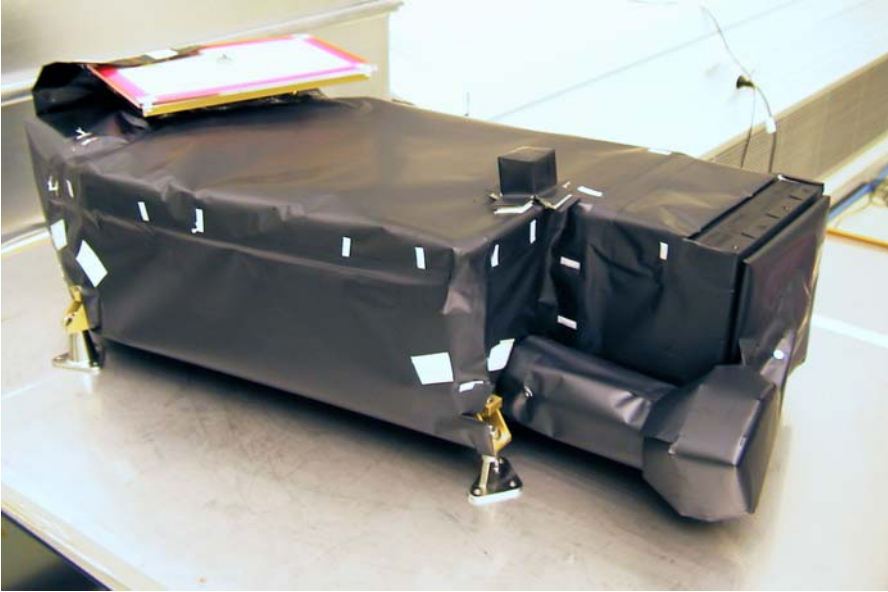
Figure 13. WAC Flight Model ready for integration.
