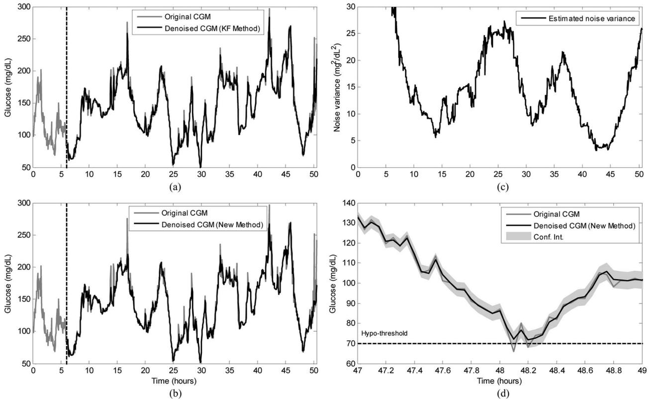
Fig. 5. Real data, subject #14. (a) and (b) CGM originally measured by the Menarini Glucoday system (gray) versus denoised CGM with KF method the new method (black) time series, respectively. The dashed vertical line indicates the time when denoising starts. (c) Estimated  $\sigma^2$  profile. (d) Zoom of time interval 47–49 h, CGM (gray) and denoised CGM with the new method (black), together with its confidence interval (gray area), time series.
