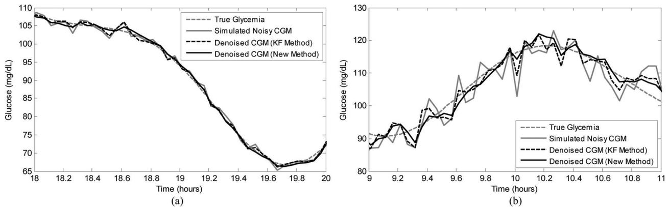
Fig. 3. Simulated study, same representative subject of Fig. 2. Panels (a) and (b) show two zooms on time intervals 18–20 h and 9–11 h, respectively. True glycemia (gray dashed), noisy simulated CGM (gray), denoised CGM with KF (black dashed) and with the new method (black) time series are displayed.
