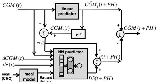
Fig. 1. Block scheme of the proposed CGM predictor.
