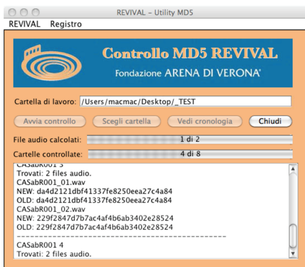
FIGURE 8: One of the software tools developed for the Fondazione Arena di Verona. This utility performs a consistency control on the checksums of the stored preservation copies and should be run periodically. The utility processes the entire archive of preservation copies and outputs a log in real-time, informing the operator about the remaining time by means of two progress bars (one for the number of preservation copies and one for the single audio files). The output on the screen reports the files that are being processed at the moment: in case of a mismatch between the checksums, an alert message is notified to the operator.
