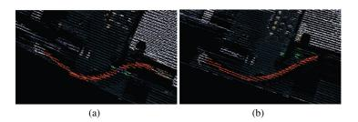
Fig. 20 Cable routing inspection using color point cloud. (a) Cable (red) correctly routed through pegs (green). (b) Incorrect cable routing.
