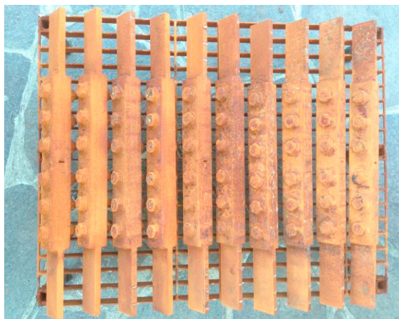
Fig. 3. a) Corroded specimens (672h); b) Mean mass losses interpolation of the corroded specimens (g/cm 2 ).
