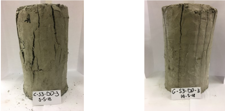
Fig. 5 Post-test cracking pattern: left, C-S3; right, G-S3.
