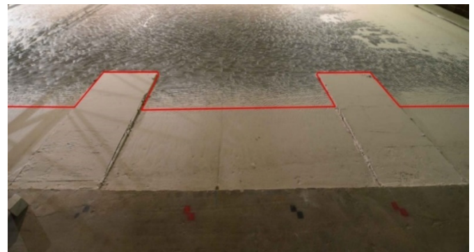
Fig. 3 "Sand groins" configuration (red line is the zero level)
