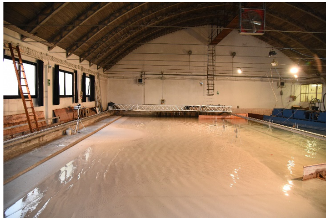
Fig. 1 The wave basin of Padova University during a wave attack
