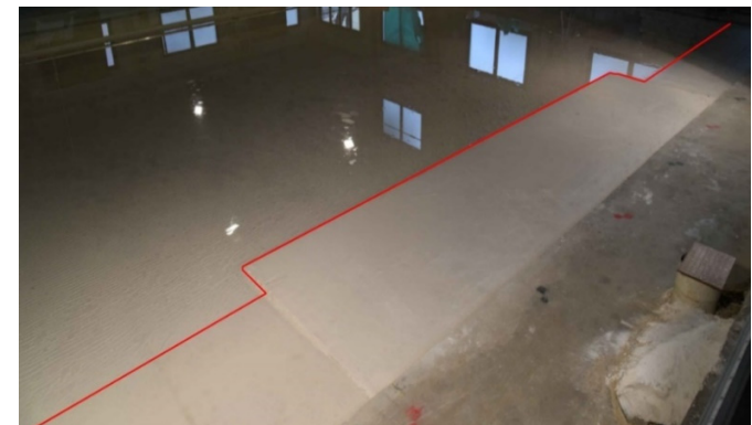
Fig. 4 Traditional nourishment configuration (red line is the zero level)
