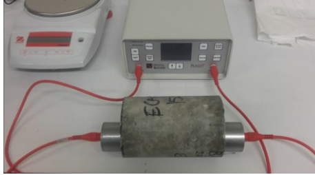
268 269 Figure 2: Ultrasonic pulse velocity apparatus for the assessment of the dynamic elastic modulus 270
