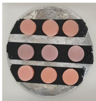
Fig. 2. The cylinder-shaped specimens from groups (CV, CAD, and 3D) used for biological investigations.
