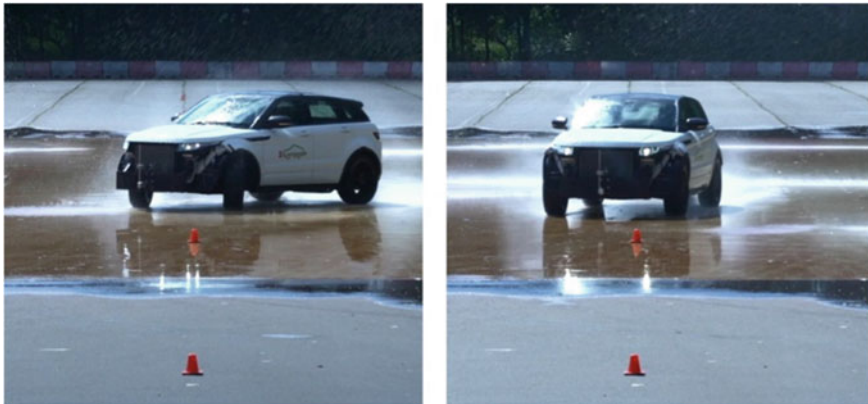
Fig. 12 A slalom test on a slippery road: (left) without controller, the driver needs to countersteer to keep the vehicle on track; (right) with controller, providing a much smoother behaviour (reproduced from Lenzo et al., 2017b)
