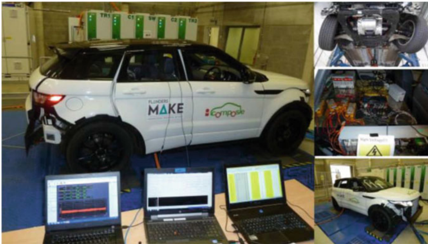
Fig. 16 The experimental setup on the rolling road facility (reproduced from Lenzo et al., 2019b)
