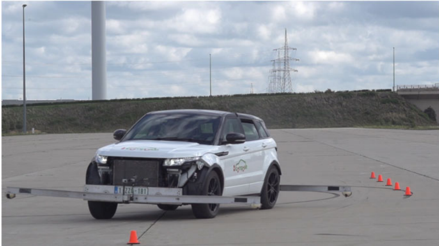
Fig. 8 The Range Rover Evoque during an obstacle avoidance manoeuvre (ISO 3888-2)
