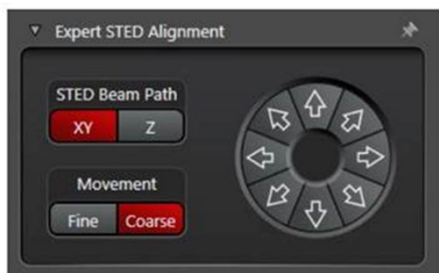
Fig.S11. “Expert STED Alignment” interface used for fine adjustments of STED beam position in the scan head. It is a customized feature activated in the Leica software and it is used to align the STED beam on the Ti:Sa remotely.
