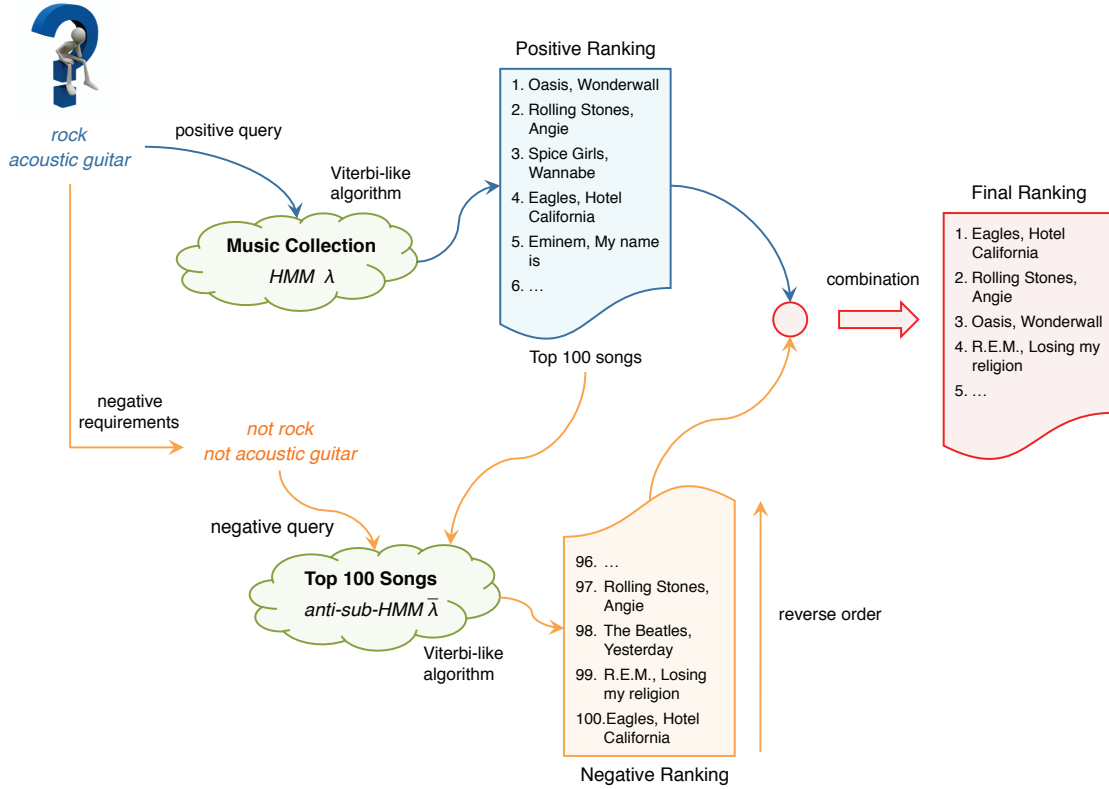
Figure 5.2. HMM-based retrieval: the user submits a query (tags or seed-song) to the system which ranks the song positively associated with the query. Later, the first positions of the list are re-ranked according to the negative information carried by the query. At the end, the system provides the user with a final ranking list obtained by combining both positive and negative results.
