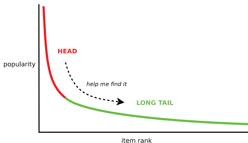
Figure 1.1. The Long Tail of items in a recommender systems: while highly popular items are also highly recommended, there is a huge quantity of less-known documents that are little ranked by state-of-the-art algorithms.
