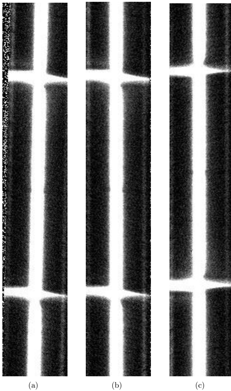
Figure 2.18: The three ordinary steps of data reduction of echelle spectra. Left: the raw spectrum, the wavelnghts increase downwards and the emission lines are tilted. Middle: the spectrum straightened in the continuum, but with the emission lines still bent. Right: the spectrum straightened and calibrated in wavelength, which changes direction (it increases upwards).
