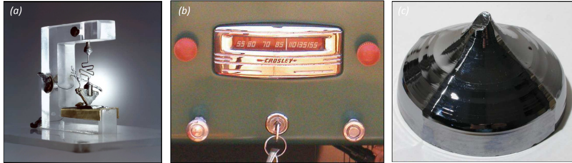
Figure 1: (a) The first transistor realized in Ge (1948); (b) early “Motorola Chrome Nose” radio Ge based; (c) Ge wafer boule.
