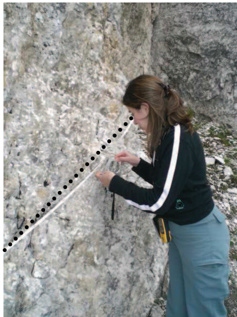
Fig. G.2. Approximate position of the oblique scanline at the basement of the northern side of the Torre Inglese pinnacle: Site 4. The trace of the scanline is drawn-in by hand. The survey was carried out from left to right over 4.00 meters.
