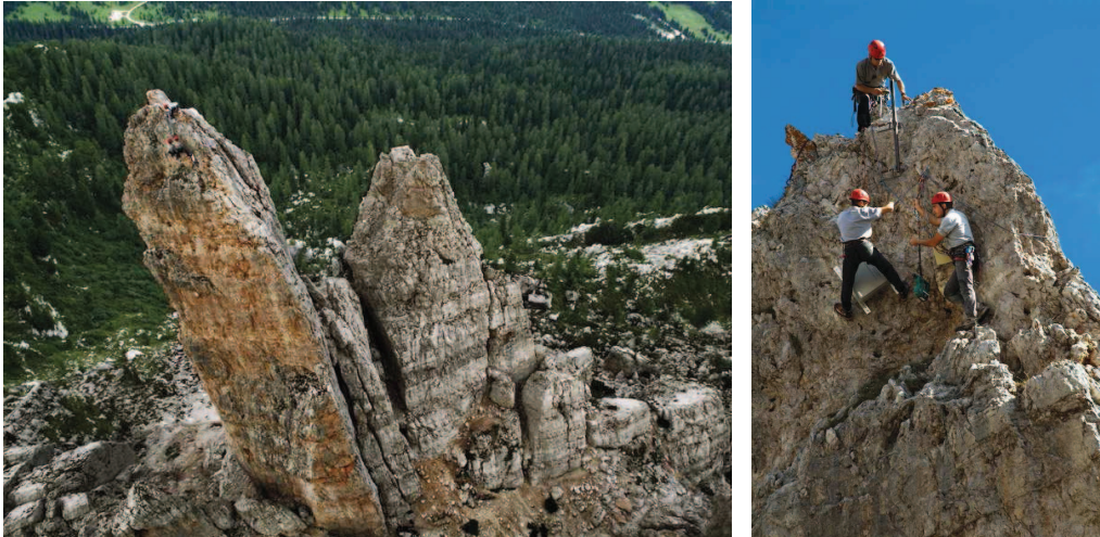
Fig. 2.3. Phases of the GPS system on the top of the Torre Inglese pinnacle. This monolith is strongly bended and presents a wide steeped discontinuity plane parallel to stratigraphy that could become a sliding surface.
