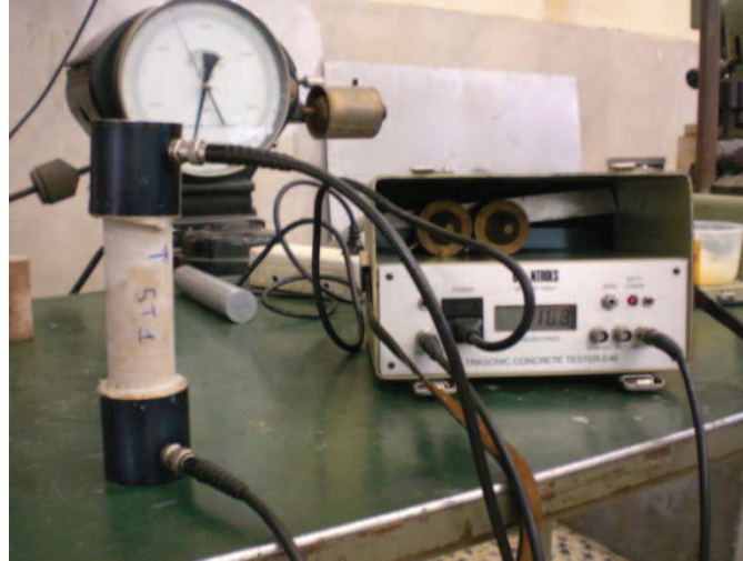
Fig. 5.7. Test equipment for ultrasonic measurements and example of specimen
