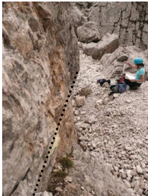
Fig. H.2. Approximate position of the oblique scanline at the basement of the northern side of the Torre Lusy pinnacle: Site 5. The trace of the scanline is drawn-in by hand. The survey was carried out from left to right over 4.85 meters.
