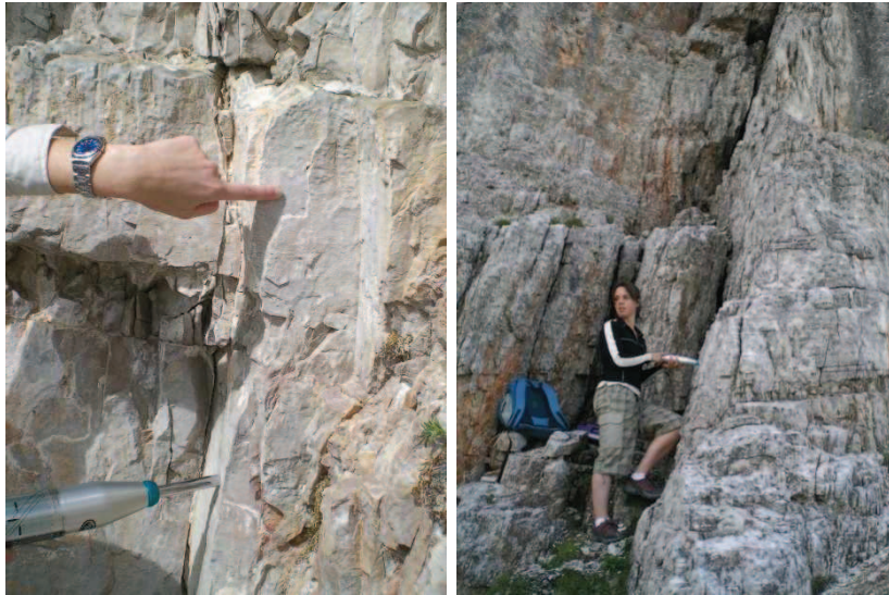
Fig. 7.8. Schmidt hammer device and types of analyzed rock discontinuities
