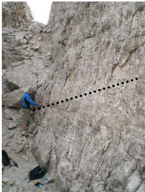
Fig. F.2. Approximate position of the oblique scanline at the basement of the northern side of the Torre Latina pinnacle: Site 3. The trace of the scanline is drawn-in by hand. The survey was carried out from left to right over 5.00 meters.
