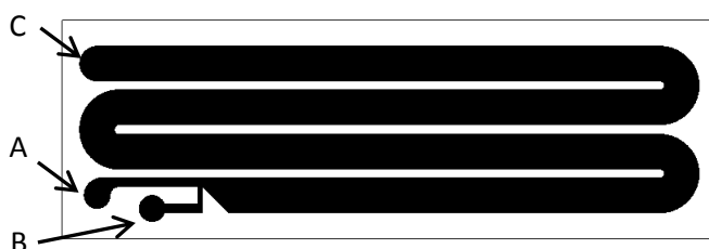
Figure 3.21. Soft photolithography mask used for the fabrication of the MFD pictured in figure 3.14. A is the inlet used for the silver colloid injection, while B was used to insufflate air for the oxygenation of the solution; C is the outlet.
