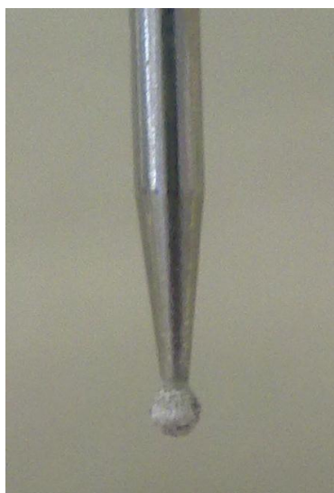
Figure 2.11. Diamond wheel point used for drilling glass plates
