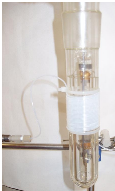
Figure 3.19. PTFE tube coiled around a photoreactor, as used for the production of AgNP seeds.
