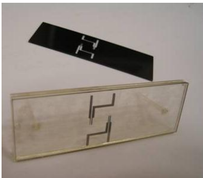
Figure 2.28. Gold electrodes sputter-coated on a glass slide. A masked slide is also pictured in the background.
