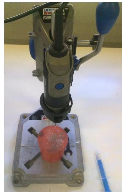
Figure 2.10. Column-mounted dremel rotary tool. A hard rubber block (red) is used to hold the glass slide during drilling.
