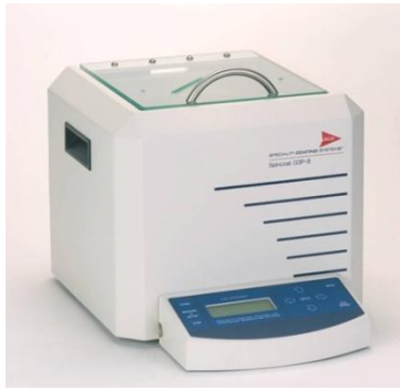
Fig. 9.11. The programmable SCS G3P-8 spin coating system used to coat our samples.
