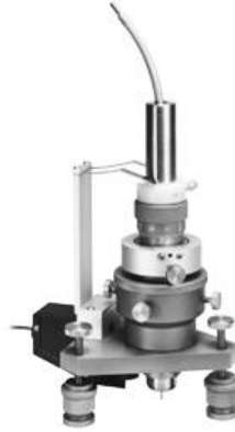
Figure 4.20: Air turbine drill - High speed air turbine drill used in the hole-drilling strain-gauge method.
