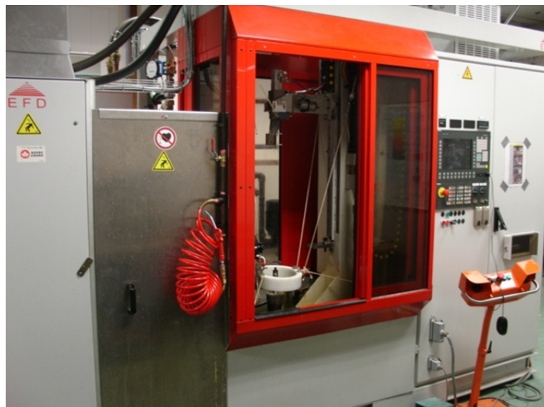
Figure 6.1: Induction equipment - Picture of the equipment used for the experimental tests.
