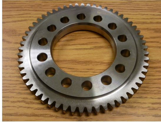
Figure 5.3: Gear test-article - Representation of the test-case used for surface hardening simulation and testing.
