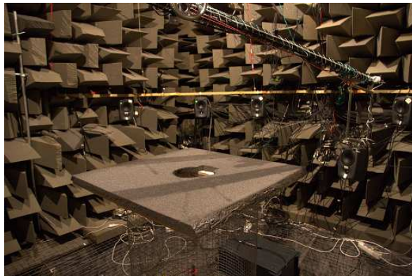
(a) The measurement setup. On bottom right, the boom-controlled loudspeaker used for sweep reproduction.
