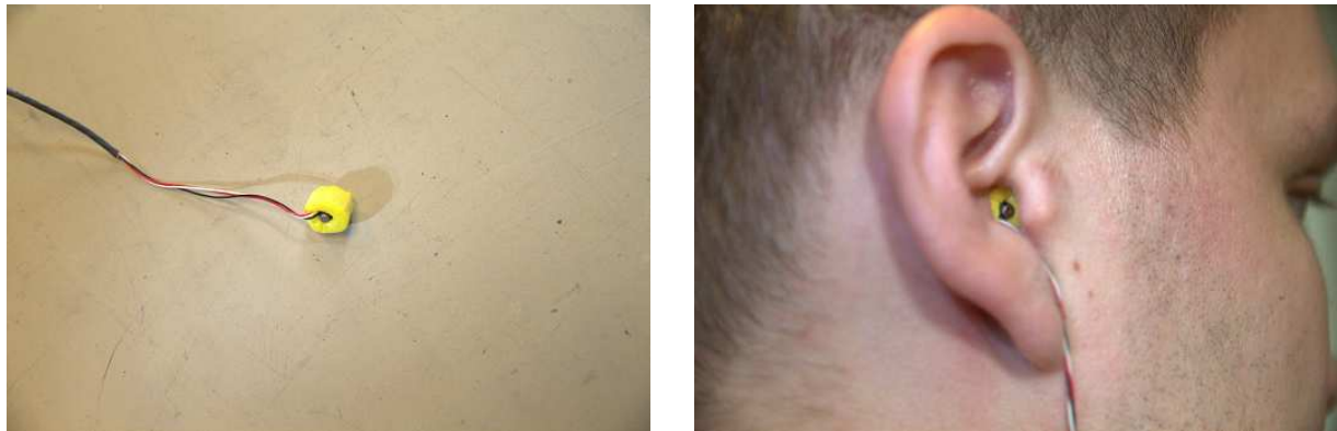
(a) Knowles FG-23329 microphone stuffed inside a hollow earplug.
