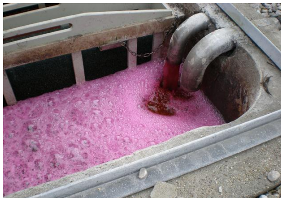
Figure 2.6 – Wastewater with rhodamine WT (RWT) tracer at sampling point (5) (influent of HF) – March 2011.
