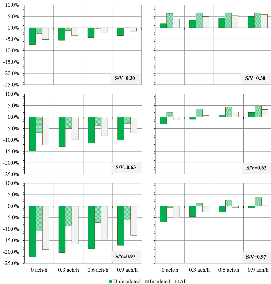
Figure 5b.3 - Percentage deviation of the simulated thermal losses with air temperature setpoint (on the left) and operative setpoint (on the right) of 26 °C respect to the losses calculated with the quasi steady state approach for different air change rates and S/V ratios
