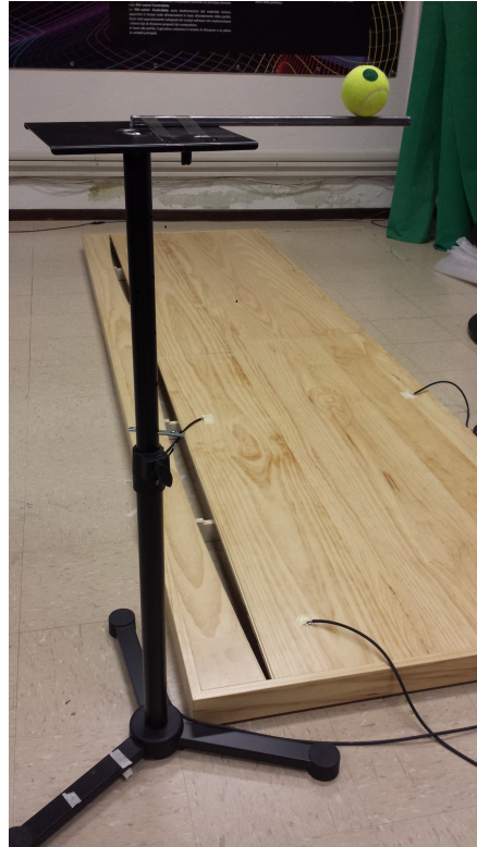
Figure 3.11: Experimental set-up: an adjustable stand for speakers, with a transverse metal bar, and a tennis ball.
