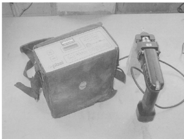
Figura 2.25 Drill energy test (RILEM TC 177-MDT.D.1)
