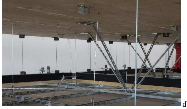
Fig. 45: Plast Sing system: a) detail of the connection between primary and secondary runners and hanger rods, b) detail of the seismic bracing system, c) placement of the seismic bracings and the hanger rods, d) specimen of Sing Plat High.
