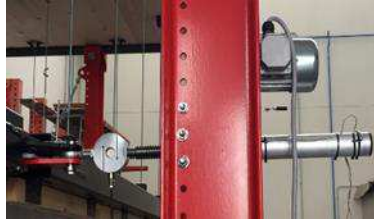
Fig. 36: Mechanical actuator and load cell.
