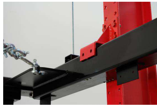
Fig. 38: a): Hinge joints connecting two tubular beams; b): brackets that guide the displacement of tubular beams.
