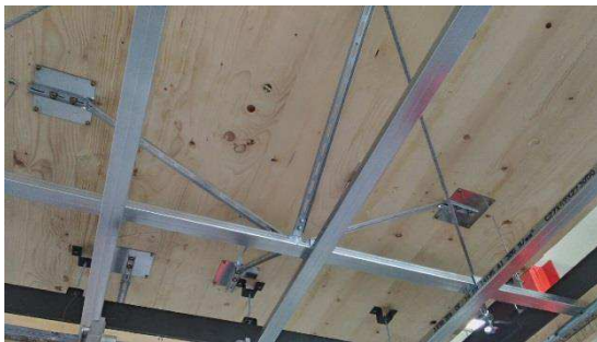
Fig. 46: Plast Doub system: a) placement of the runners and the plasterboards and details of the bracket and the hanger rods, b) picture of the installation of primary and secondary runners, c) installation of the seismic bracing system, d) picture of a specimen.
