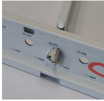
Fig. 20: Detail of damage on M-M Stand B15 specimen: tearing of the slot in the transversal runner.
