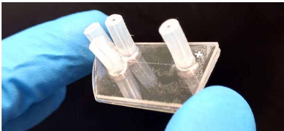
Figure 2.1. the picture report an example of a lithium niobate chip, where a droplet generator circuitry is engraved by mean of a self-polishing saw technique, as described in [7].
