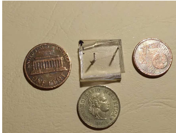
Figure 2.5. \text{LiNbO}_3 optofluidic device sealed with a cover of PDMS by means of oxygen plasma treatment. The fluidic connections in this case have been done using 1 mm outer diameter steel capillary.
