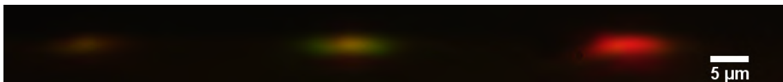
Figure 4.36. Example of the waveguides outputs, where a broadband in the visible range was coupled into the input waveguide, and due to the relation dispersion of the liquid inside the channel, each spectral component has different d , and so it is coupled in different output waveguide of the pattern.
