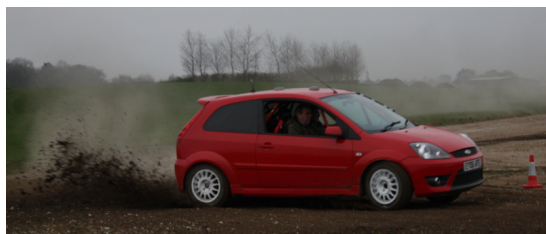
Figure 3.24: FWD test vehicle driven by a professional driver during data collection on a loose off-road surface.
