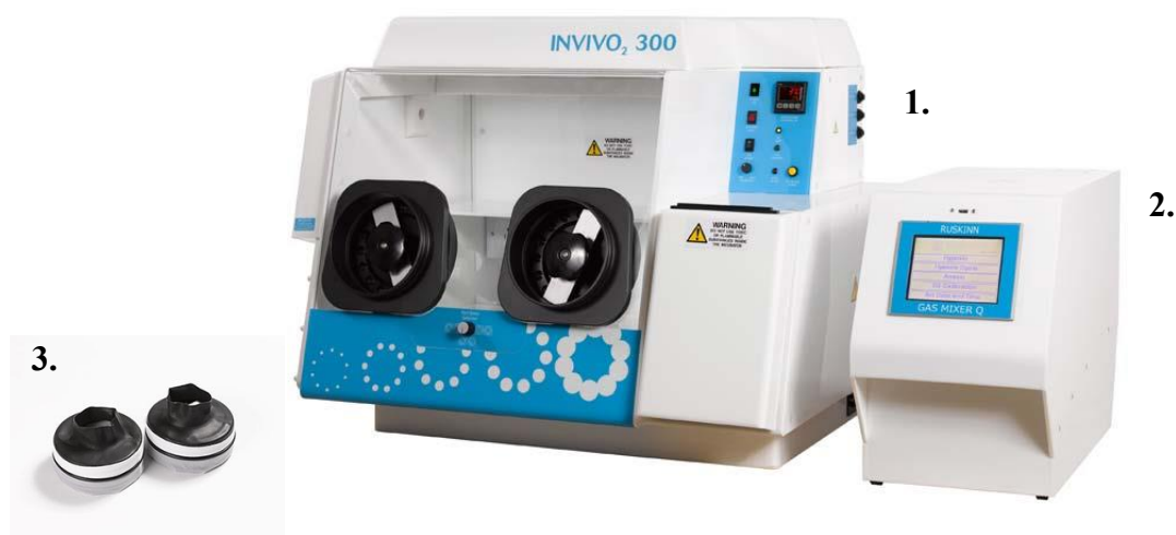
Figure 12: The Invivo2 300 Hypoxia Workstation (Ruskinn C300). The system is provided of a chamber for maintaining cultures (1.); a gas mixer Q (2.) and a glove box (3.). In our experiments it has been programmed to observe 2% O 2 , 5% CO 2 , 93% N 2 gas levels balance.
