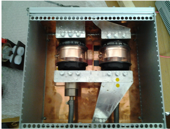
Figure 3.6: Picture of the inside of the matching box: two variable in-vacuum capacitor are used. All the connections are made by copper plates to exploit the skin effect.
