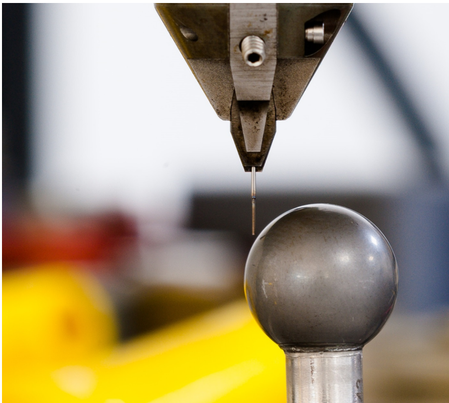
Figure 5.1: Image of a 10 mm steel sphere being measured on the \mu EDM machine with a 0.2 mm cylindrical tool-probe.
