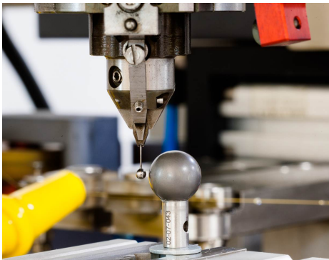
Figure 5.11: Image of the 2 mm spherical probe clamped on the Sarix SX-200 spindle, while approaching the 10 mm reference sphere.
