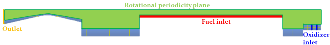
Figure 2.19: Numerical investigation about vortex: boundary conditions
