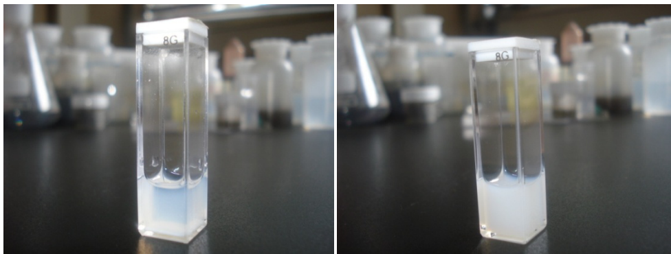
Figure 2.7: Static (left) and agitated (right) samples of POE+TiO 2 0.1 wt%
