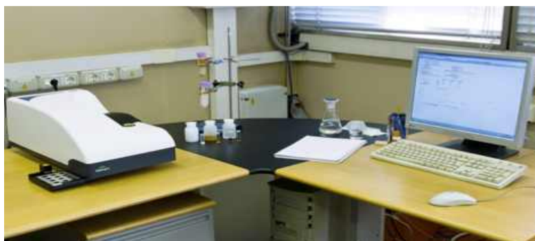
Figure 2.6: Zetasizer Nano ZS (Malvern) used to measure nanoparticles dimension
