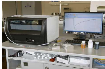
Figure 2.9: Thermtest TPS 2500 S (Hot Disk) for thermal conductivity measurements
