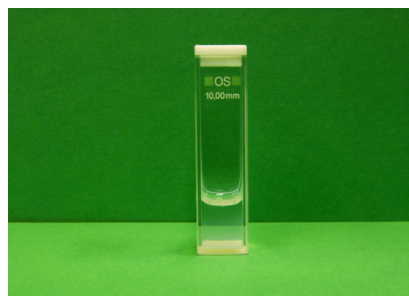
Figure 2.5: Unstable nano-oil prepared with continuous sonication technique
