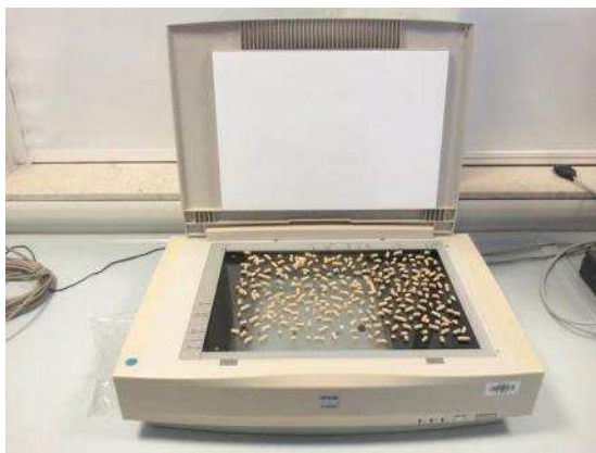
Figure 6-2: RGB scanner (left) and the taken image (right)
