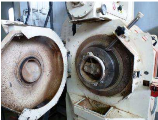
Figure 5-4: the pellet press CLM200 open (left) and in operation (right)
