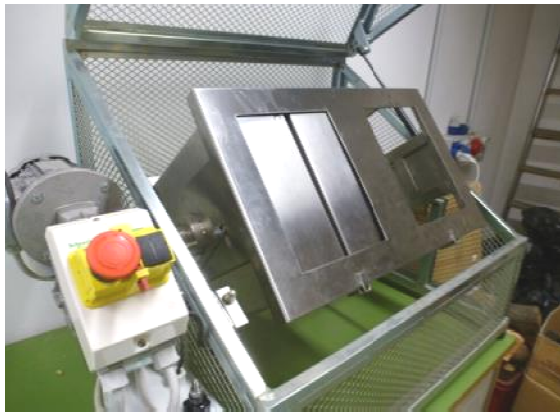
Figure 4-1: pellet durability tester
