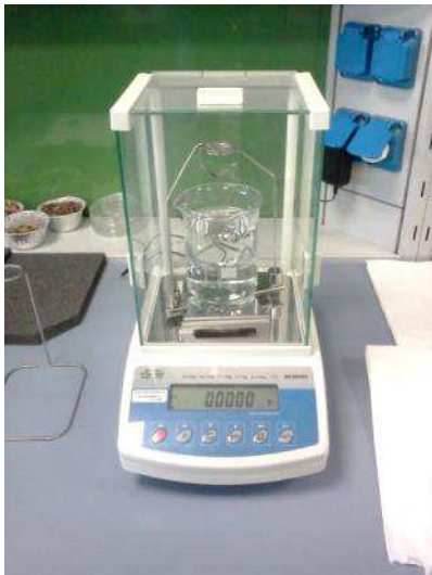
Figure 4-3: instrument for determination of the particle density of pellets
