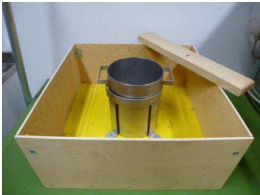
Figure 4-2: apparatus to measure the bulk density
