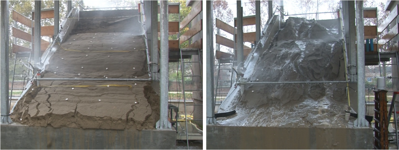
Figure 4-11. Images of the sand layer after failure in the two experiments: with loose sand one on the left and dense sand one on the right.
