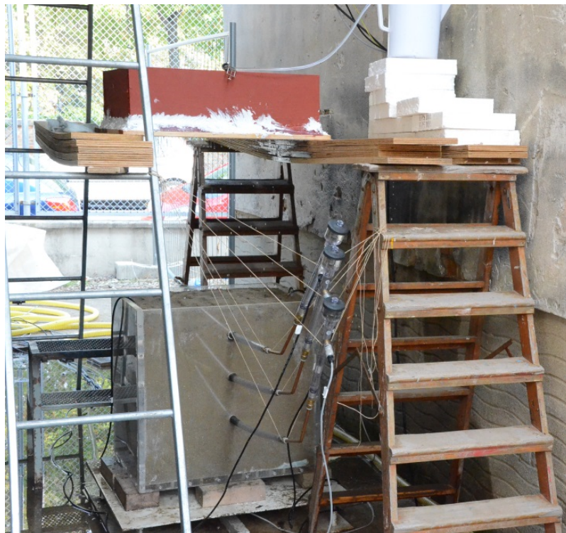
Figure 3-2. Experimental device used for the calibration of the WCR probes
