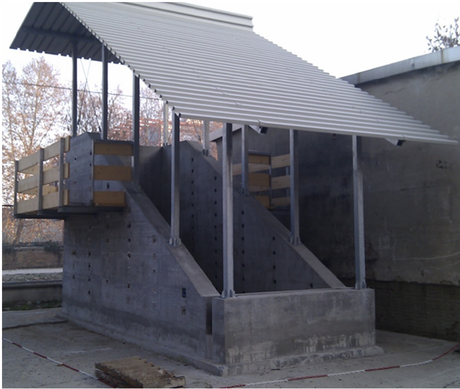
Figure 1-1. The artificial hillslope model.
