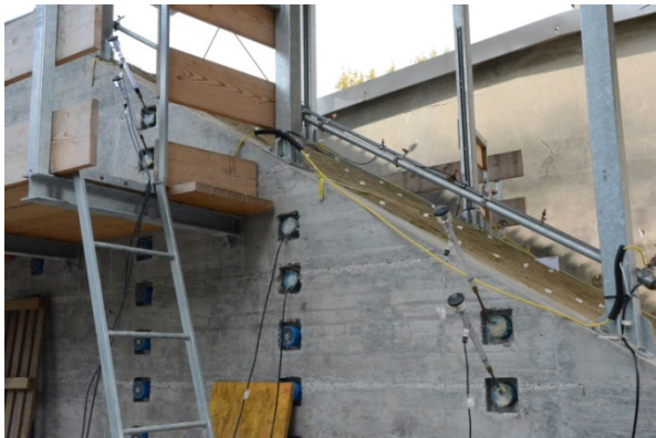
Figure 4-3. A view on lateral side of the hillslope model: tensiometers are arranged in the top soil by means of the holes applied in the walls.
