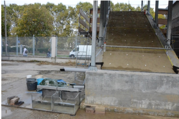
Figure 4-2. V-notch gauge located at the slope toe
