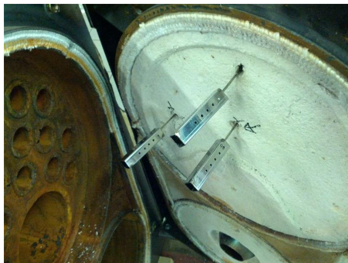
Figure 1.2.1.3. Picture of the shielded thermocouples located at the inlet of the third pass.
