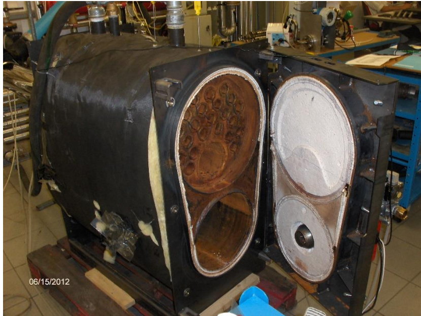
Figure 1.2.1.2. Photo of the heat generator (opened) used for the experimental analysis.
