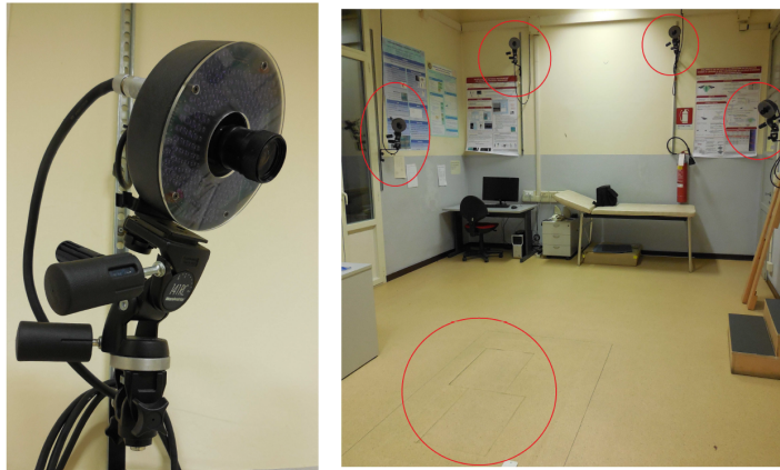
Figure 35: Equipments of the Bioengineering of the Movement Laboratory . The four frontal cameras are circled as well as the force plates. Besides, the detail of the camera is shown.
