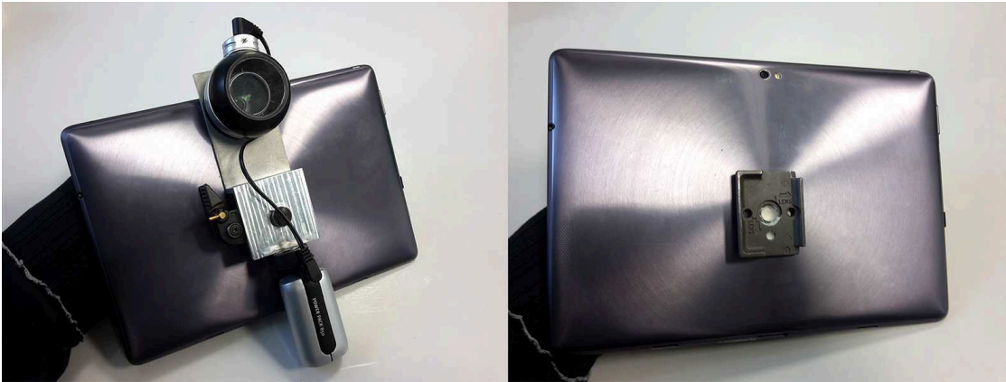
Figure 32: The DermLite FOTO mounted on the ASUS Transformer Prime using the prototype lens mount (left), and the part of the mount that is always attached to the tablet (right).
