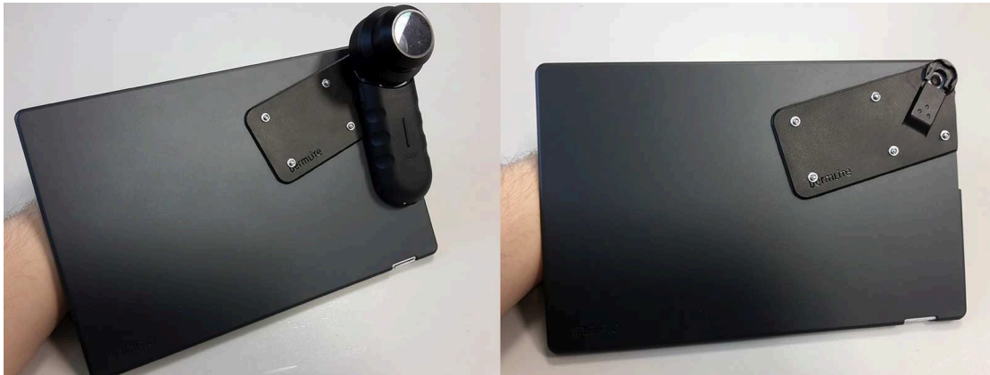
Figure 33: The DermLite DL3 mounted on the Sony Xperia Tablet Z using the updated prototype lens mount (left), and the part of the mount that is always attached to the tablet (right).
