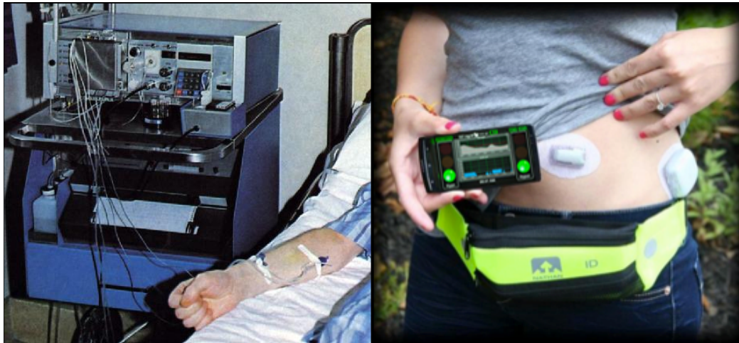
Figure 1.2: Technology evolution in AP research: the Biostator [11] ( Left panel ); a portable AP in 2010s, i.e. Diabetes Assistant (DiAs) [40] ( Right panel ).
