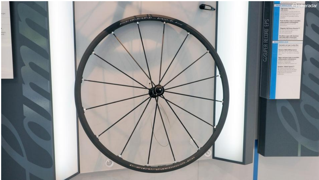
Fig.1.22 PEO treated rim with Keronite process
