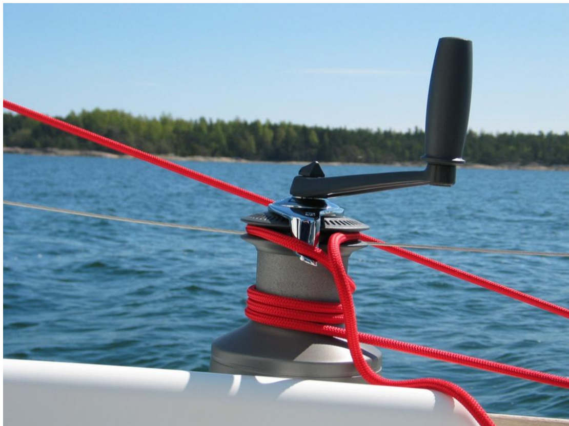
Fig.1.23 PEO coated yacht winch drum
