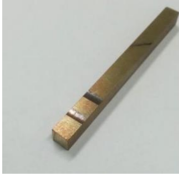
Fig.2.9 Sample after the wear test
