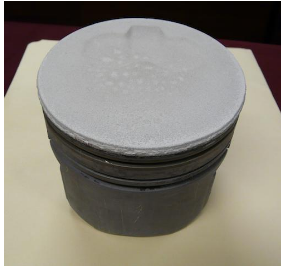
Fig.1.24 PEO process applied on a gear and on a piston head
