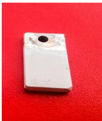
Fig. 1.16 PEO treated sample of AZ91 magnesium alloy
