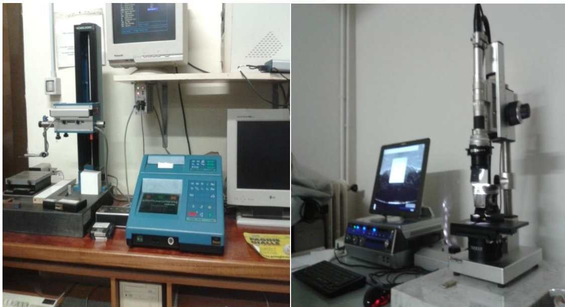
Fig.2.10 Profilometer (on the left) and multifocal microscope (on the right) used for the characterization of the samples after the wear tests.
