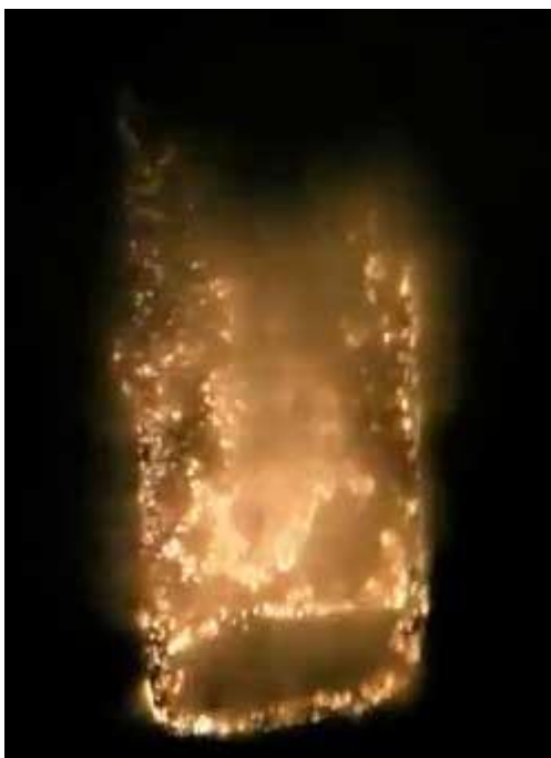
Fig. 1.4 Typical discharges formed during PEO process
