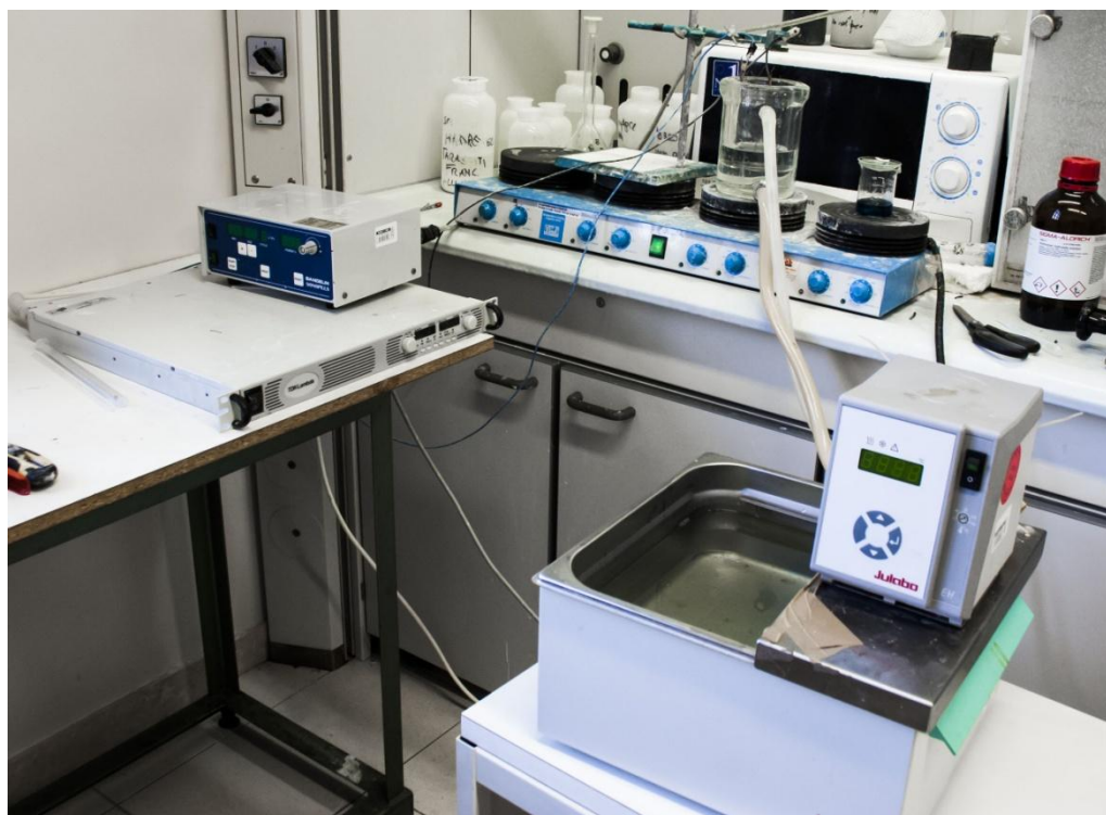
Fig.2.2 Laboratory system used to produce PEO coatings.
