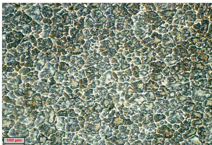
Fig. 4.11 Microstructure of 7075 alloy
