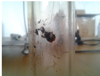
FIGURE 5.8: Perforation of the discharge chamber wall: the damage is limited to a relatively small hole, surrounded by a zone showing signs of thermal stress. This was interpreted as a sign of an electric arc between the plasma and the antenna.
