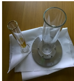
FIGURE 5.15: The existing discharge chamber (left), developed for HPH.Com and characterized by an inner diameter of 19 mm, and the new one (right).
