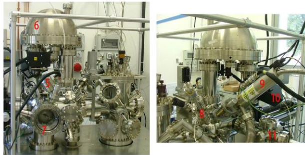
A. Preparation Chamber (UHV: 5.0 \cdot 10^{-9} mbar, RHK Technology UHV-750) B. STM/AFM Chamber (UHV: 6.5 \cdot 10^{-11} - 1.0 \cdot 10^{-10} mbar, RHK Technology UHV-750 / SPM1000)
