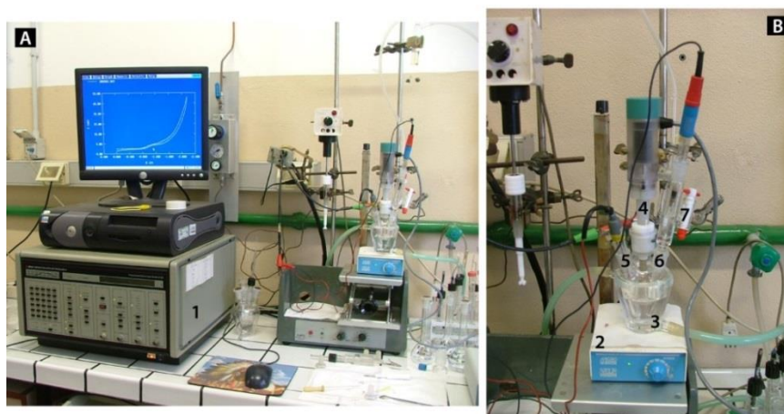
Figure 3.3. Experimental equipment for electrochemical tests; a: whole equipment (1: potentiostat); b: electrochemical cell with thermostatic bath (2: stirrer, 3: four cones cell, 4: RDE-WE, 5: Pt-CE, 6: RE, 7: Ar inlet for the outgas of the electrolyte).
