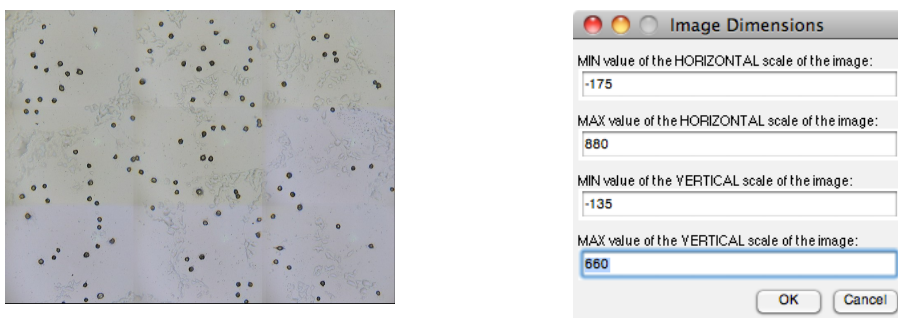
Figure 4.18: At the left, a typical image usable with COF5. On the right, the coordinates and dimension of the sample are introduced. Into this example, the image extends by more than 1mm in length and about 0.8 mm in height.
