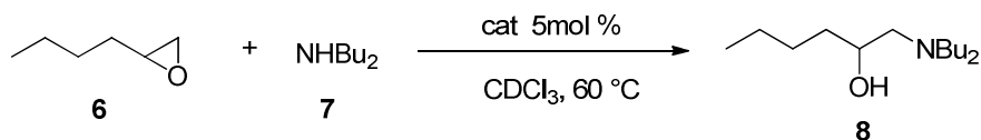
Scheme 3 Reaction conditions used for catalysts screening in epoxide ring opening reaction of 1,2-epoxyhexane 6 by dibutylamine 7 .
