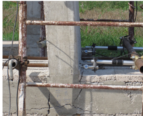
Figure 11-8. Specimen 9 at failure
