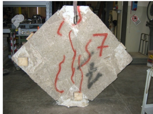
Figure 9-14. Cracks at failure of panel n.7
