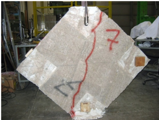
Figure 9-15. failure of panel n.7
