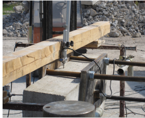
Figure 11-6. Vertical sensor for vertical displacements
