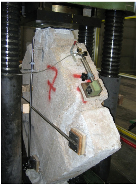
Figure 9-9. Instrumentation (panel left side)
