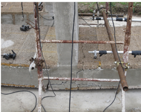
Figure 11-9. Specimen 10 at failure
