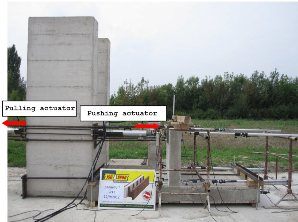
Figure 11-4. Actuators used during the tests on connections
