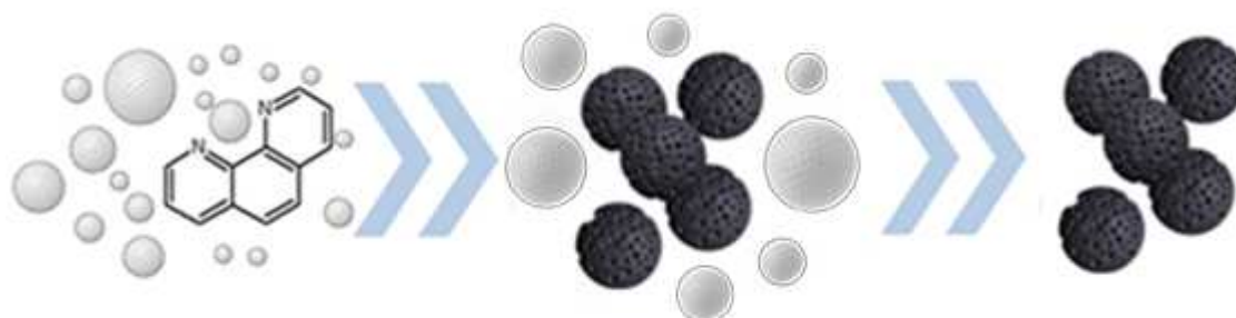
Figure 1.17 Hard template process for mesoporous carbon synthesis: mixing of inorganic template and carbon precursor, followed by pyrolysis and chemical etching of the template.
