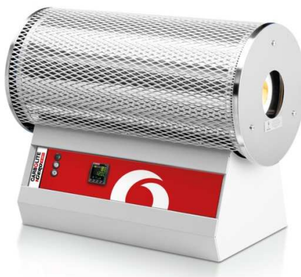
Figure 4.3 Tubular oven used for the pyrolysis step during the synthesis of mesoporous carbons.
