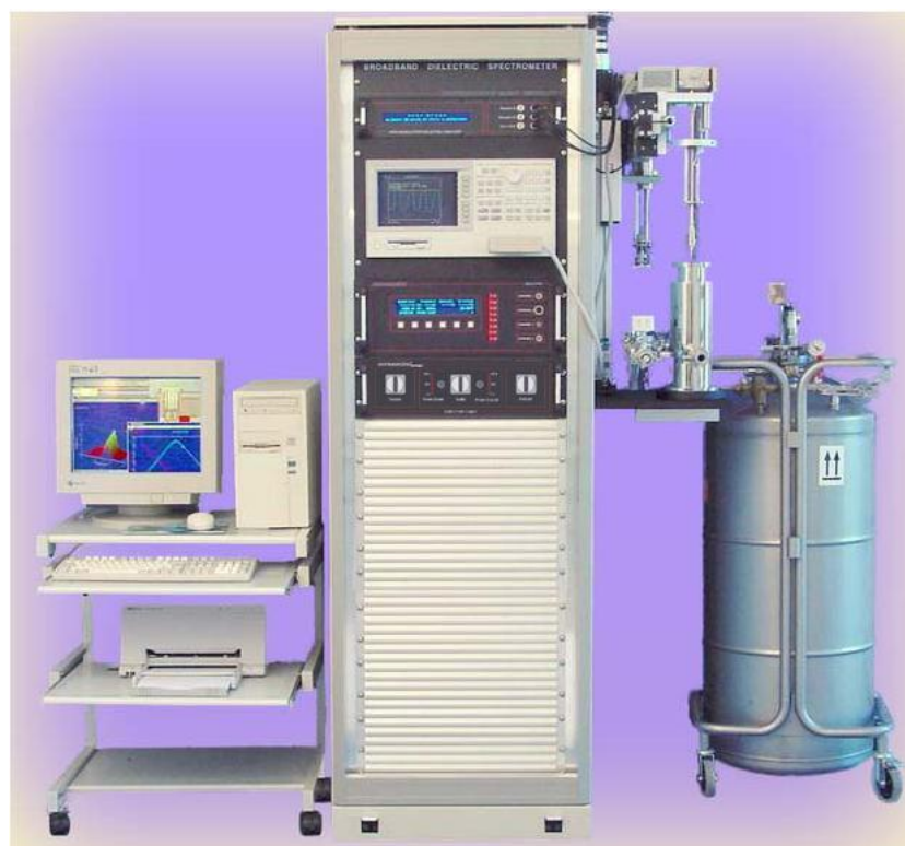
Figure 2.3 BES measuring system including the analyzer, temperature control system, the cryostat and sample holder cell, vacuum pump (hidden) and electronic data management.
