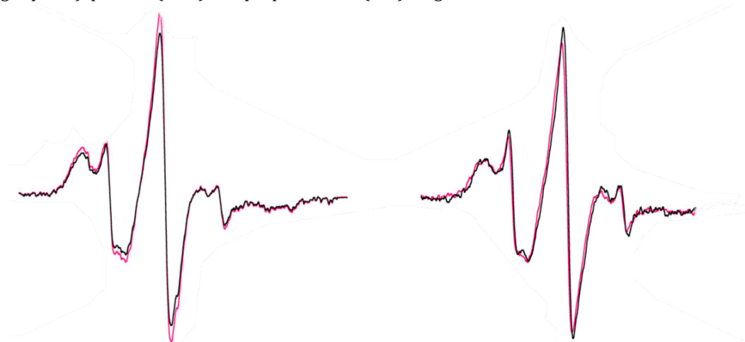
RLC-31 labelled with MSL spin probe. Rigor buffer (left panel) and relax ATP blebbistatin buffer (right panel), perpendicular (black) and parallel (red) magnetic field.
