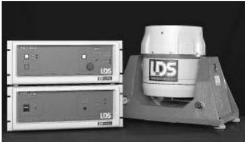
Fig. 15: the shaker LDS 650 and the amplifier 1000 PA.
