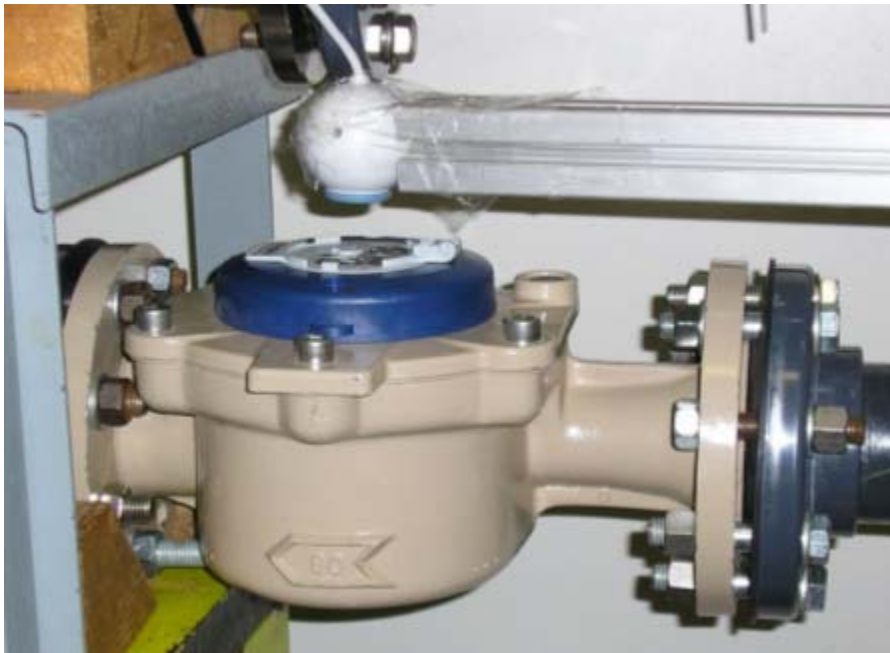
Fig. 8: the webcam is located over the display of the meter.
