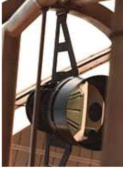
Figure 2.8: The secondary mirror at the "Copernico" telescope.
