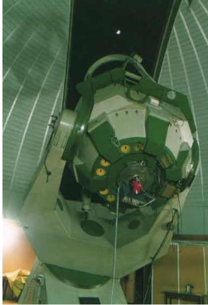
Figure 2.9: The "Copernico" Cassegrain focus.
